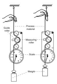
If this procedure shows a deviation beyond the allowable tolerance and a reliable operation is no longer allowed, the instrument has to be recalibrated or repaired.
